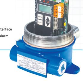
All calibration and power wiring is done at the main control unit. This is mounted directly onto the probe.
